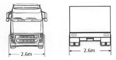
**Note:** Side cargo overhangs from the two sides of the vehicle cannot exceed 30cm.
